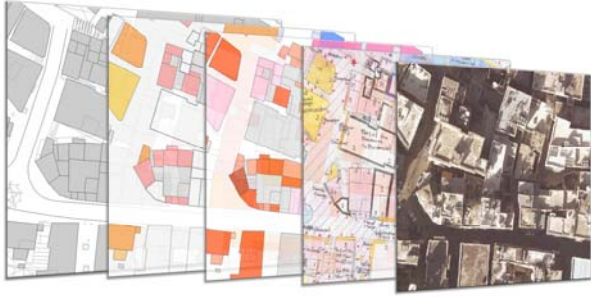
6. The interactive cartography overlap different thematic layers such as functions, number of floors, site surveys, aerial photos, historic cartography, etc.
